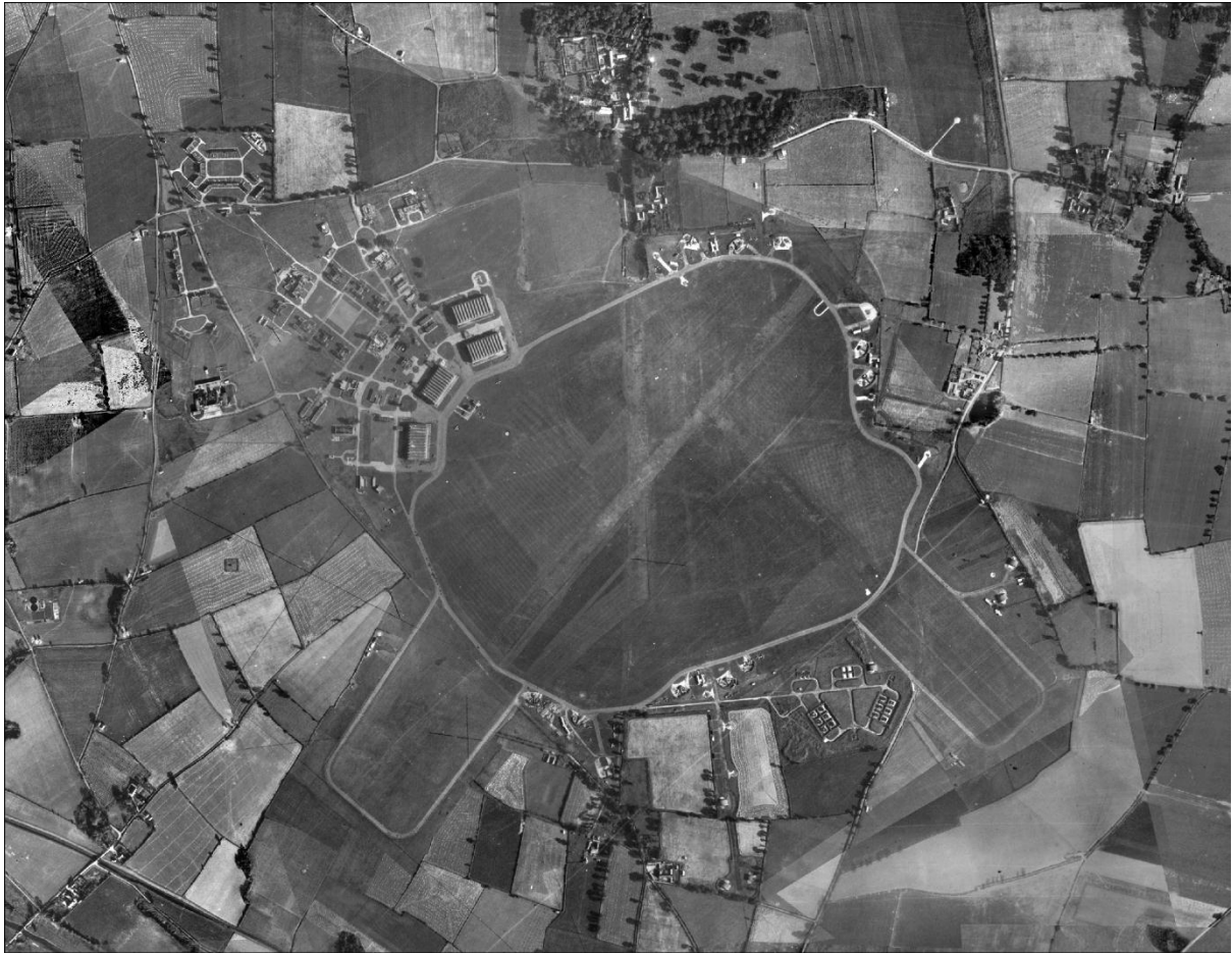
Figure 12: 1946 Aerial view of RAF Coltishall showing Expansion Period Design of married quarters, technical and domestic area to the north-west. Note the grassed World War Two runways and the dispersal pens around the perimeter to the north and south.
